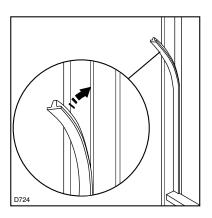
Apply covers (B) on joint cover lugs and into hinge holes.
